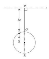
A thin uniform rod PQ has mass m and length 3a. A thin uniform circular disc, of mass m and radius a, is attached to the rod at Q in such a way that the rod and the diameter QR of the disc are in a straight line with PR = 5a. The rod together with the disc form a composite body, as shown in the figure. The body is free to rotate about a fixed smooth horizontal axis L through P, perpendicular to PQ and in the plane of the disc.
