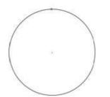
M.I. of hoop about perpendicular axis through its centre =  $mr^2 \leftarrow$ =  $1.2 \times 1.5^2$  kg m<sup>2</sup>
