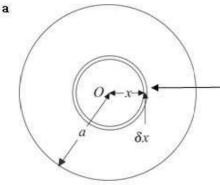
You consider the disc as made up a series of concentric rings of thickness  $\delta x$ . The area of each ring is  $2\pi x \delta x$ .
