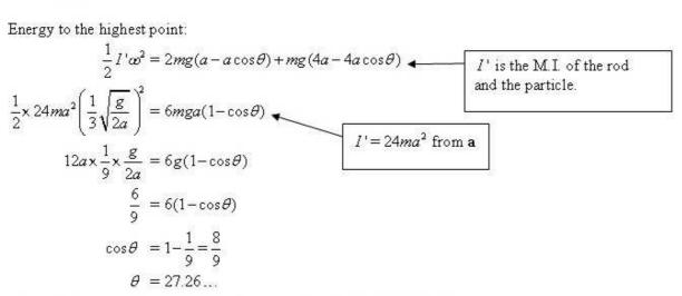
The angle between the rod and the downward vertical is 27.3" (3s.f.)
