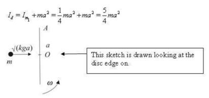
Let the angular velocity of the disc and P immediately after impact be  $\omega$ . Conservation of angular momentum about A
