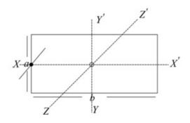
Take XX', YY' and ZZ' as three axes meeting at O, the centre of the rectangle. XX' and YY' are parallel to sides of the rectangle and ZZ' is perpendicular to the rectangle.
