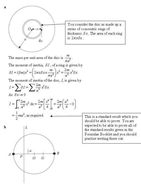
The moment of inertia of the disc about L is given by
