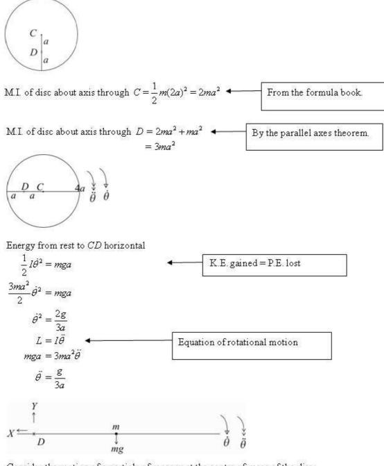
Consider the motion of a particle of mass *m* at the centre of mass of the disc:
