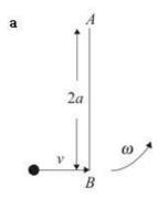
Let the angular speed of the rod immediately after the impact be  $\omega$ . The moment of inertia, *I*, of the rod combined with the particle about *A* is given by
