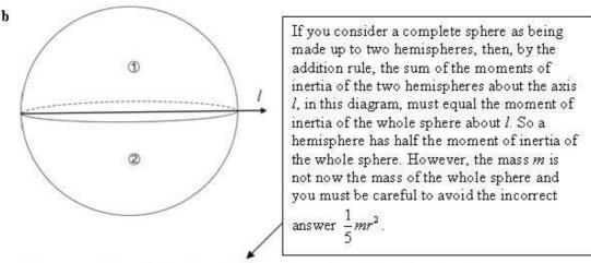
If the mass of the whole sphere is 2m and the radius of the sphere is r, then using the result of part **a**, the moment of inertia of the whole sphere is
