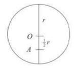
Let O be the centre of the disc and the point where the axis of rotation meets the disc be A. By the parallel axes theorem, the moment of inertia,  $I_A$ , of the disc about A is given by
