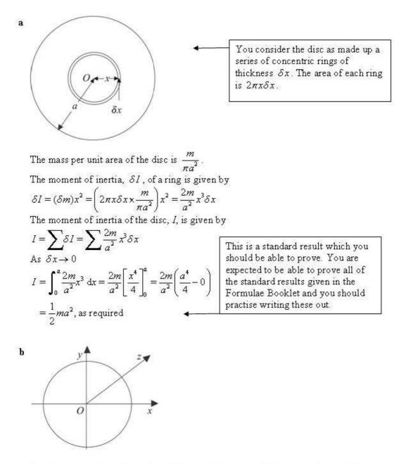
Let the centre of the disc be O and Ox and Oy be perpendicular axes through O. By the perpendicular axes theorem, the moment of inertia,  $I_{Ox}$ , about a diameter Ox through O is given by
