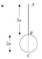
The moment of inertia of the rod about the axis through A is given by
