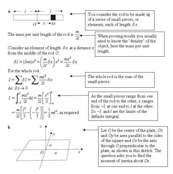
By the stretching rule, the moment of inertia of the lamina about Ox and Oy is given by
