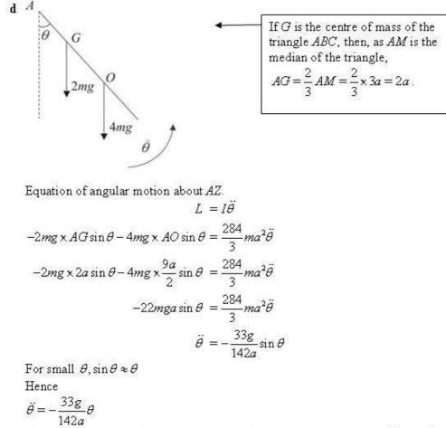
Comparing with the standard equation for simple harmonic motion,  $\ddot{\theta} = -\omega^2 \theta$ , the motion is approximately simply harmonic, with  $\omega^2 = \frac{33g}{142a}$ . The period of small oscillations is given by
