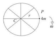
M.I. of flywheel and particle about given axis through C
