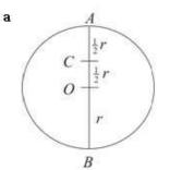
Let the centre of the disc be O. By the parallel axes theorem, the moment of inertia,  $I_C$ , of the disc about C is given by
