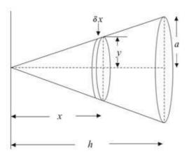
You consider the cone to be made up of thin discs, each of thickness  $\delta x$  with the centre of the disc at a distance x from the vertex of the cone. If the radius of the disc is y, then, using the formula,  $V = \pi r^2 h$ , for the volume of a cylinder, the volume of a thin disc is  $\pi y^2 \delta x$ .
