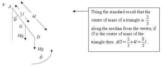
The moment of inertia, I, of the triangle about a smooth horizontal axis through A perpendicular to the plane of the triangle is given by
