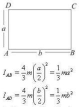
$\therefore$  Moment of inertia about an axis through A perpendicular to the
