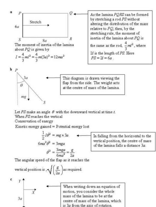
Let the magnitude of the vertical component of the resultant force of the axis PQ on the flap, as it reaches the vertical position be Y.
