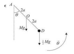
The moment of inertia of the compound pendulum, I, about the axis through A is given by
