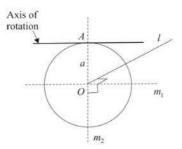
By symmetry, the moments of inertia about the perpendicular axes  $m_1$  and  $m_2$ , shown in the diagram, are equal.
