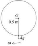
M.I. of disc + particle about axis through  $O = \frac{1}{2} \times 20 \times (0.5)^2 + 4 \times (0.5)^2$ = 3.5 kg m<sup>2</sup>
