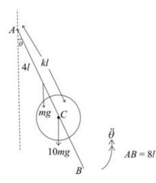
M.I. of rod and disc about axis at A
