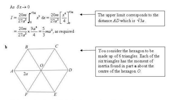
The hexagon is made up of 6 triangles of mass m, where M = 6m. The moment of inertia of the hexagon about an axis through  $O, I_0$ , is given by
