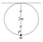
Moment of inertia of sphere about diameter =  $\frac{2}{5}(2m)a^2$
