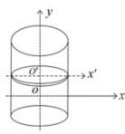
Take the y-axis as the axis of the cylinder and the x-axis passes through the centre of gravity as shown.
