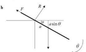
Using the standard formula for the moment of inertia of a rod about its centre  $\frac{1}{3}ml^2$  with l = 2a. The centre of mass of the rod is the distance a from the edge of the table.
