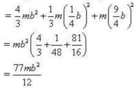
Use the parallel axes theorem for CDEF. Remember to move from the centre of mass.
