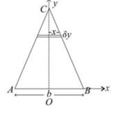
Divide the triangle into strips. The one shown has mass  $2x\delta y \times \rho$
