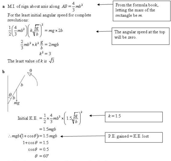
: BC makes an angle of 60° with the upward vertical.
