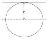
Moment of inertia about a diameter  $=\frac{2}{5}mr^2$ Then using parallel axes theorem: Moment of inertia about tangent  $=\frac{2}{5}mr^2 + mr^2$  $=\frac{7}{5}mr^2$
