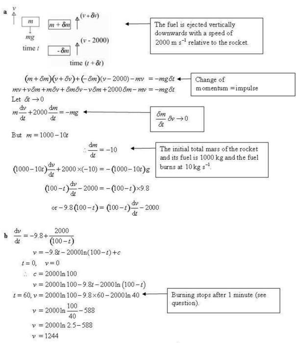
When burning stops, the speed of the rocket is  $1200 \text{ m s}^{-1}$  (2 s.f.)
