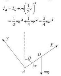
When AO has rotated through an angle  $\theta$ , let the components of the force parallel and perpendicular to AO be X and Y respectively. Conservation of energy
