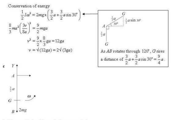
Let the magnitude of the vertical component of the force acting on the rod at A immediately after the impact be Y.
