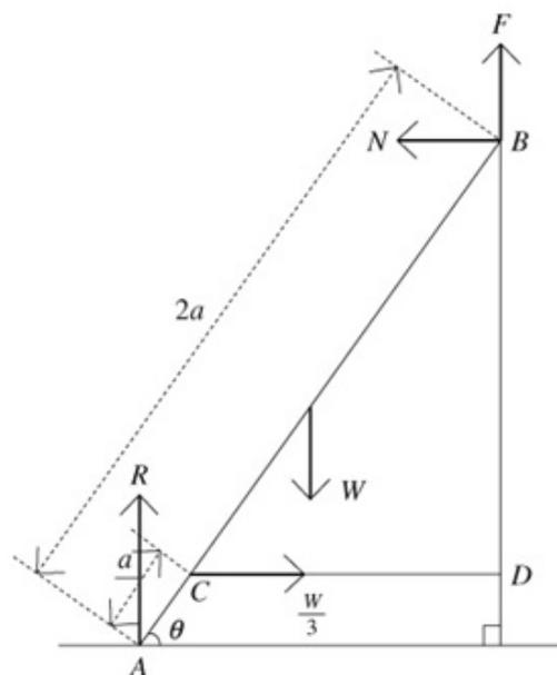
Let  $R$  be the normal reaction at  $A$ ,  $N$  the normal reaction at  $B$  and  $F$  the friction at  $B$ .
