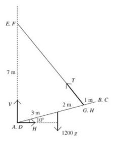
V and H are the vertical and horizontal components of the force at the hinge. T is the tension in the cables.
