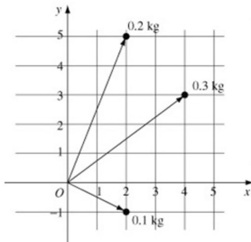
This diagram illustrates the positions of the particles with respect to Cartesian axes. You take moments about the  $y$ -axis and the  $x$ -axis to find the  $x$ - and  $y$ -coordinates, respectively, of the centre of mass of the system of particles.
