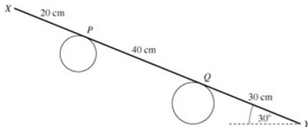
A uniform rod  $XY$  has weight  $20\text{ N}$  and length  $90\text{ cm}$ . The rod rests on two parallel pegs, with  $X$  above  $Y$ , in a vertical plane which is perpendicular to the axes of the pegs, as shown in the diagram. The rod makes an angle of  $30^\circ$  to the horizontal and touches the two pegs at  $P$  and  $Q$ , where  $XP = 20\text{ cm}$  and  $XQ = 60\text{ cm}$ .
