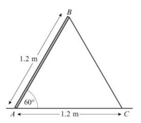
A trap door is propped open at 60° to the horizontal by a pole. The trap door is modelled as a uniform rod AB, of mass 10 kg and length 1.2 m, smoothly hinged at A. The pole is modelled as a light rod BC, smoothly hinged to AB at B. The points A and C are at the same horizontal level, AC = 1.2 m and the plane ABC is vertical, as shown in the diagram.
