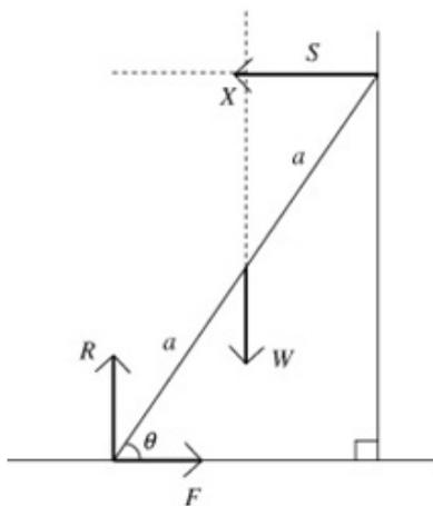
Suppose that the ladder has length  $2a$  and weight  $W$ .
