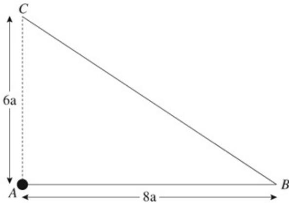
A uniform rod  $AB$ , of length  $8a$  and weight  $W$ , is free to rotate in a vertical plane about a smooth pivot at  $A$ . One end of a light inextensible string is attached to  $B$ . The other end is attached to point  $C$  which is vertically above  $A$ , with  $AC = 6a$ . The rod is in equilibrium with  $AB$  horizontal, as shown in the diagram.
