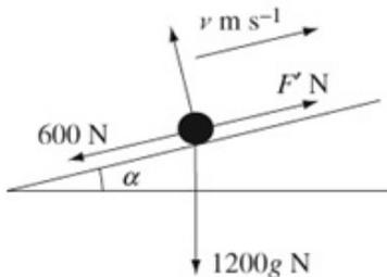
Let the speed of the car be  $u \text{ m s}^{-1}$  and the driving force of the engine have magnitude  $F' \text{ N}$ .
