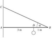
The girder is modelled as a rod, and the cables as light inextensible strings.
