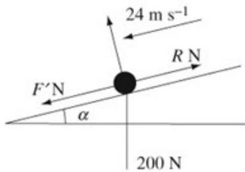
Let  $F'$  N be the magnitude of the driving force produced by the engine of the model car as it moves downhill.
