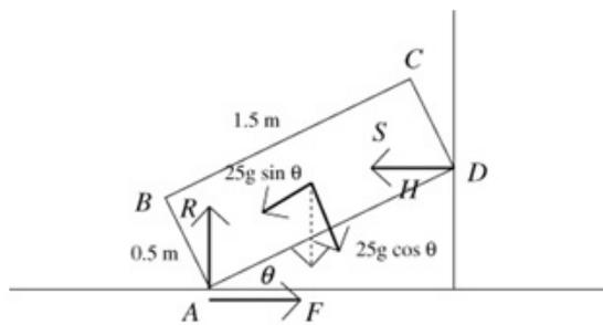
$R$  and  $S$  are the normal reactions at  $A$  and  $D$  respectively.  $F$  is the friction at  $A$ .
