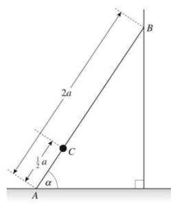
A uniform ladder AB, of mass m and length 2a, has one end A on rough horizontal ground. The other end B rests against a smooth vertical wall. The ladder is in a vertical plane perpendicular to the wall. The ladder makes an angle  $\alpha$  with the horizontal, where  $\tan \alpha = \frac{4}{3}$ . A child of mass 2m stands on the ladder at C where  $AC = \frac{1}{2}a$ , as shown in the diagram. The ladder and the child are in equilibrium.
