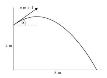
A ball is thrown from a point 4 m above horizontal ground. The ball is projected at an angle  $\alpha$  above the horizontal, where  $\tan \alpha = \frac{3}{4}$ . The ball hits the ground at a point which is a horizontal distance 8 m from its point of projection, as shown in the figure above. The initial speed of the ball is  $u \text{ m s}^{-1}$  and the time of flight is T seconds.
