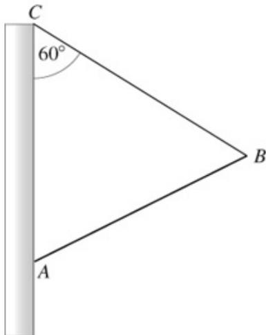
A uniform rod  $AB$  of mass  $m$  rests in equilibrium with  $A$  in contact with a rough vertical wall. The coefficient of friction between the rod and the wall is  $\mu$ . A light string is attached to  $B$  and to a point  $C$  of the wall, where  $C$  is vertically above  $A$ . The plane  $ABC$  is perpendicular to the wall,  $BC = BA$  and  $\angle ACB = 60^\circ$ , as shown in the diagram.
