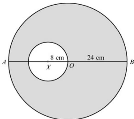
The figure shows a template  $T$  made by removing a circular disc, of centre  $X$  and radius  $8$  cm, from a uniform circular lamina, of centre  $O$  and radius  $24$  cm. The point  $X$  lies on the diameter  $AOB$  of the lamina and  $AX = 16$  cm. The centre of mass of  $T$  lies at the point  $G$ .
