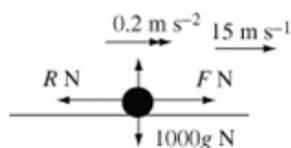
a Let  $F$  N be the magnitude of the driving force produced by the engine of the car.
