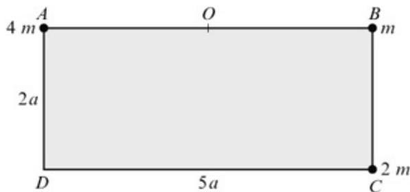
A loaded plate  $L$  is modelled as a uniform rectangular lamina  $ABCD$  and three particles. The sides  $CD$  and  $AD$  of the lamina have length  $5a$  and  $2a$  respectively and the mass of the lamina is  $3m$ . The three particles have mass  $4m$ ,  $m$  and  $2m$  and are attached at the points  $A$ ,  $B$  and  $C$  respectively, as shown in the figure.
