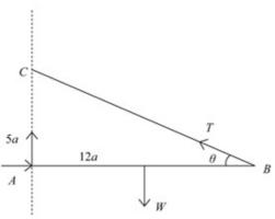
Let the angle between the string and the rod be  $\theta$ , T be the tension in the string, X the horizontal component of the force at A and Y the vertical component of the force at A.
