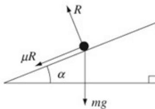
Let the normal reaction between the particle and the plane have magnitude  $R$  N.
