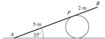
Find the normal and frictional components of the contact force at  $A$ , and hence find the least possible value of the coefficient of friction between the ladder and the ground.
