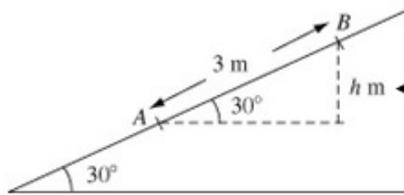
The change in the potential energy of  $P$  depends on the vertical distance it has moved. You find this using trigonometry.
