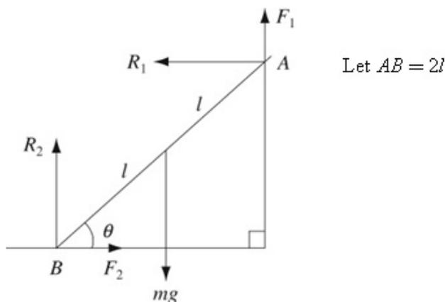
$$F_1 = \mu_1 R_1 \quad F_2 = \mu_2 R_2$$
