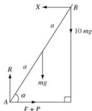
**a**  $M(A) \quad X \times 2a \sin \alpha = 10mg \times 2a \cos \alpha + mg \times a \cos \alpha$
