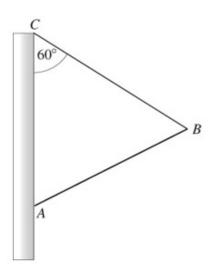
A uniform rod AB of mass *m* rests in equilibrium with A in contact with a rough vertical wall. The coefficient of friction between the rod and the wall is  $\mu$ . A light string is attached to B and to a point C of the wall, where C is vertically above A. The plane ABC is perpendicular to the wall, BC = BA and  $\angle ACB = 60^{\circ}$ , as shown in the diagram.
