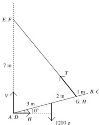
$V$  and  $H$  are the vertical and horizontal components of the force at the hinge.
