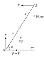
**a** M(A)  $X \times 2a \sin \alpha = 10 mg \times 2a \cos \alpha + mg \times a \cos \alpha$  $2X \tan \alpha = 20 mg + mg$
