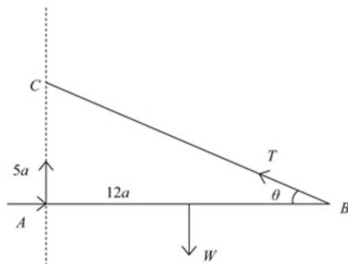
Let the angle between the string and the rod be  $\theta$ ,  $T$  be the tension in the string,  $X$  the horizontal component of the force at  $A$  and  $Y$  the vertical component of the force at  $A$ .
