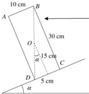
The greatest value which  $\alpha$  can take without toppling about  $D$  corresponds to the situation where the centre of plate, here labelled  $O$ , is vertically above  $D$ . As drawn here, if  $O$  was to the left of  $D$ , the weight of the plate would have an anticlockwise moment about  $D$  and the plate would rotate about  $D$ .
