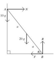
N is the normal reaction at A, R is the normal reaction at B, and F is the frictional force at B.
