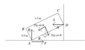
R and S are the normal reactions at A and D respectively. F is the friction at A.
