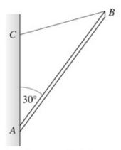
A uniform rod AB of mass m and length 2a is smoothly hinged to a vertical wall at A and is supported in equilibrium by a rope which is modelled as a light string. One end of the rope is attached to the end B of the rod and the other end is attached to a point C of the wall, where C is vertically above A, AC = CB, and  $\angle CAB = 30^\circ$ , as shown in the diagram.
