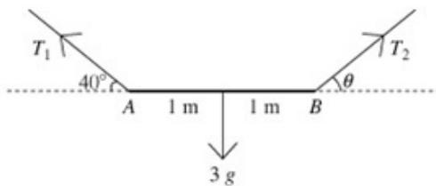
$$M(B) \quad T_1 \times \sin 40^\circ \times 2 = 3g \times 1$$
