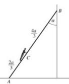
By modelling the ladder as a rod and the child as a particle, calculate the least possible value of the coefficient of friction between the ladder and the ground.
