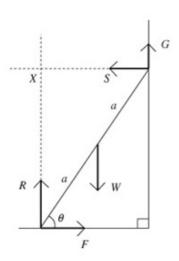
R and F are the normal reaction and the friction where the ladder is in contact with the ground. S and G are the normal reaction and the friction at the wall.
