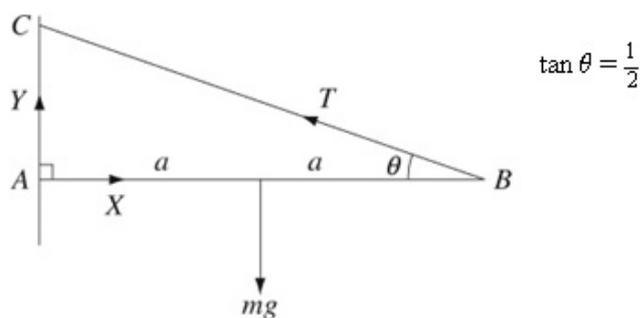
a  $M(A) \quad T \times 2a \sin \theta = mg \times a$  ← Take moments about  $A$  for an equation with  $T$  as the only unknown quantity.
