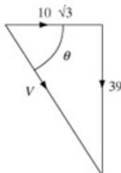
$$\begin{aligned} V^2 &= u_x^2 + v_y^2 \\ &= (10\sqrt{3})^2 + (-39)^2 = 1821 \\ V &= \sqrt{1821} = 42.673\dots \\ \tan \theta &= \frac{39}{10\sqrt{3}} \Rightarrow \theta \approx 66.05^\circ \end{aligned}$$
