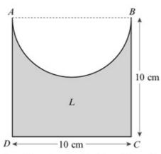
A uniform lamina L is formed by taking a uniform square sheet of material ABCD of side 10 cm and removing a semicircle with diameter AB from the square, as shown in the figure.
