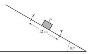
A small package is modelled as a particle P of mass 0.6 kg. The package slides down a rough plane from a point S to a point T, where ST = 12 m. The plane is inclined at 30° to the horizontal and ST is a line of greatest slope of the plane, as shown in the figure. The speed of P at S is 10 m s<sup>-1</sup> and the speed of P at T is 9 m s<sup>-1</sup>. Calculate
