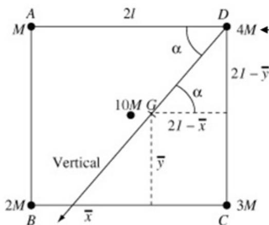
The angle required in c is marked  $\alpha$  in the diagram. It has been brought into a right angled triangle, in which you can use trigonometry, using alternate (Z) angles.
