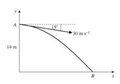
A stone is thrown from a point A with speed 30 m s<sup>-1</sup> at an angle of 15° below the horizontal. The point A is 14 m above horizontal ground. The stone strikes the ground at the point B, as shown in the figure above. Find
