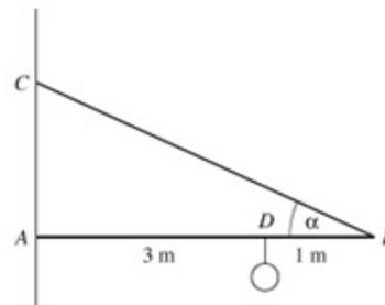
The girder is modelled as a rod, and the cables as light inextensible strings.
