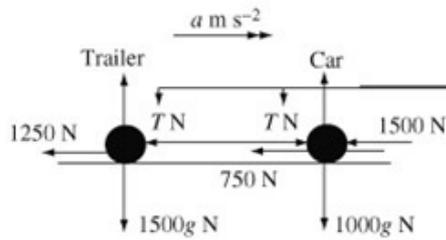
Let the acceleration of the car while braking be  $a \text{ m s}^{-2}$ .
