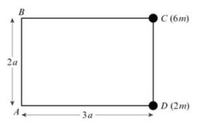
The figure shows four uniform rods joined to form a rectangular framework ABCD, where AB = CD = 2a and BC = AD = 3a. Each rod has mass *m*. Particles of mass 6*m* and 2*m* are attached to the framework at points *C* and *D* respectively.
