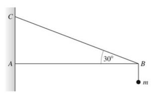
A uniform rod AB has mass 2m and length a. The end A is smoothly hinged at a fixed point. A particle of mass m is suspended from the rod at the end B. The loaded rod is held in equilibrium in a horizontal position by a light string, one end of which is attached to the rod at B, the other end being fixed to a point C vertically above A, as shown in the diagram. The string makes an angle of 30° with the horizontal.
