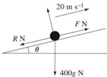
Let  $F\text{N}$  be the magnitude of the driving force produced by the engine.
