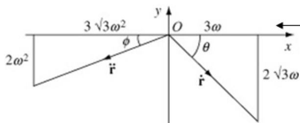
A diagram is essential here. Once the diagram has been drawn, the problem reduces to basic trigonometry. You find the angles using the inverse tangent button on your calculator. The final angle could be given in degrees or radians ( $1.92^\circ$ ).
