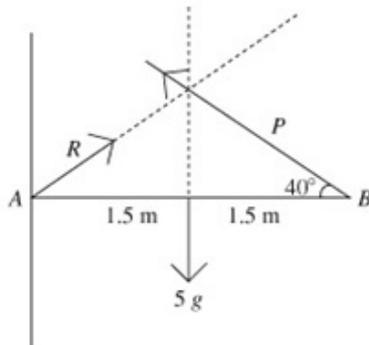
Because the rod is uniform we know that the centre of mass is at the mid-point of the rod. This implies a symmetrical diagram (isosceles triangle), so we know that  $R$  acts at  $40^\circ$  to the rod and the magnitudes of  $P$  and  $R$  are equal.
