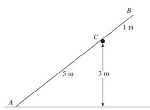
A smooth horizontal rail is fixed at a height of 3 m above a horizontal playground whose surface is rough. A straight uniform pole AB, of mass 20 kg and length 6 m, is placed to rest at a point C on the rail with the end A on the playground. The vertical plane containing the pole is at right angles to the rail. The distance AC is 5 m and the pole rests in limiting equilibrium as shown in the diagram. Calculate
