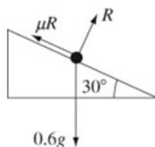
Let the normal reaction between the particle and the plane have magnitude  $R$  N.
