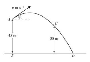
A particle P is projected from a point A with speed  $u \text{ m s}^{-1}$  at an angle of elevation  $\theta$ , where  $\cos \theta = \frac{4}{5}$ . The point B, on horizontal ground, is vertically below A and AB = 45 m. After projection, P moves freely under gravity passing through a point C, 30 m above the horizontal ground, before striking the ground at the point D, as shown in the figure above.
