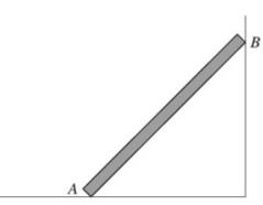
The diagram shows a uniform heavy plank of wood AB, of mass m, whose lower end A is resting on rough horizontal ground and whose upper end B is resting against a rough vertical wall. The coefficient of friction between the plank and the ground and
