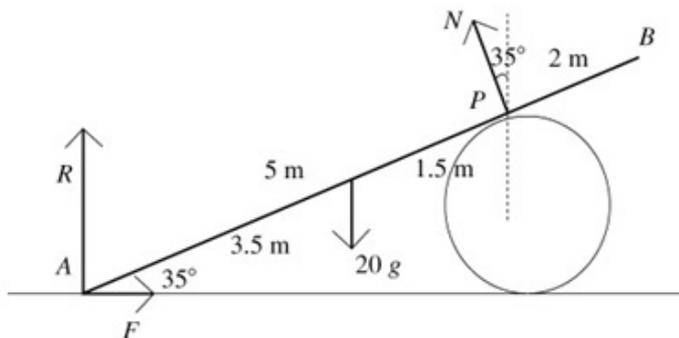
$N$  is the normal reaction at  $P$ ,  $R$  is the normal reaction at  $A$  and  $F$  is the friction at  $A$ .
