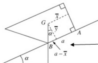
When the lamina is on the point of overturning about  $B$ , the centre of mass  $G$  of the lamina is vertically above  $B$ .
