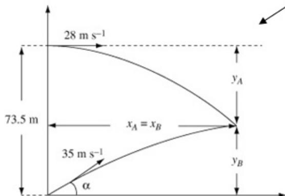
It helps you to draw a sketch to illustrate the data of the question. This shows that, for  $A$  and  $B$  to collide, two conditions have to be met. Firstly, the horizontal distances moved by  $A$  and  $B$  (here labelled  $x_A$  and  $x_B$ ) have to be equal. Secondly the distance fallen by  $A$  ( $y_A$ ) and the distance moved upwards by  $B$  ( $y_B$ ) must add up to the height of the cliff, 73.5 m.
