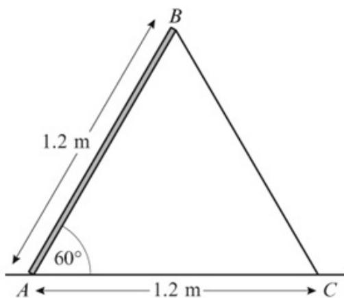
A trap door is propped open at  $60^\circ$  to the horizontal by a pole. The trap door is modelled as a uniform rod  $AB$ , of mass 10 kg and length 1.2 m, smoothly hinged at  $A$ . The pole is modelled as a light rod  $BC$ , smoothly hinged to  $AB$  at  $B$ . The points  $A$  and  $C$  are at the same horizontal level,  $AC = 1.2$  m and the plane  $ABC$  is vertical, as shown in the diagram.
