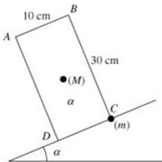
The greatest value of  $\alpha$  occurs when the centre of mass, say  $G$ , of the plate combined with the stud is vertically above  $D$ . The first step in this part must, therefore, be finding the position of  $G$ .
