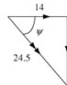
$\psi$  can now be found using trigonometry. There is no need to find the vertical component of the velocity at  $C$ .
