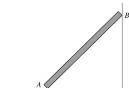
The diagram shows a uniform heavy plank of wood  $AB$ , of mass  $m$ , whose lower end  $A$  is resting on rough horizontal ground and whose upper end  $B$  is resting against a rough vertical wall. The coefficient of friction between the plank and the ground and between the plank and the wall is  $\frac{2}{3}$ .
