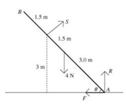
S is the normal reaction at C, R is the normal reaction at A, and F is the friction at A.  $\theta$  is the angle between the pole and the ground.
