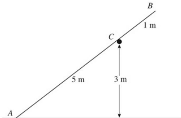
A smooth horizontal rail is fixed at a height of 3 m above a horizontal playground whose surface is rough. A straight uniform pole  $AB$ , of mass 20 kg and length 6 m, is placed to rest at a point  $C$  on the rail with the end  $A$  on the playground. The vertical plane containing the pole is at right angles to the rail. The distance  $AC$  is 5 m and the pole rests in limiting equilibrium as shown in the diagram. Calculate
