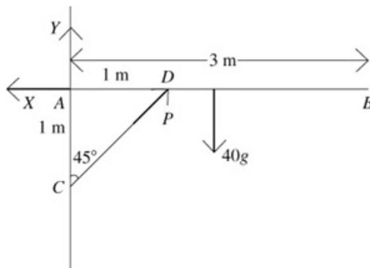
Let the horizontal and vertical components of the force at  $A$  be  $X$  and  $Y$  respectively. Let the thrust in the rod be  $P$ .
