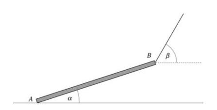
A straight log AB has weight W and length 2a. A cable is attached to one end B of the log. The cable lifts the end B off the ground. The end A remains in contact with the ground, which is rough and horizontal. The log is in limiting equilibrium. The log makes an angle  $\alpha$  to the horizontal, where  $\tan \alpha = \frac{5}{12}$ . The cable makes an angle  $\beta$
