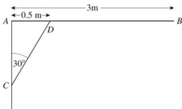
A uniform pole  $AB$ , of mass 30 kg and length 3 m, is smoothly hinged to a vertical wall at one end  $A$ . The pole is held in equilibrium in a horizontal position by a light rod  $CD$ . One end  $C$  of the rod is fixed to the wall vertically below  $A$ . The other end  $D$  is freely jointed to the pole so that  $\angle ACD = 30^\circ$  and  $AD = 0.5$  m, as shown in the diagram. Find
