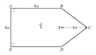
The figure shows a uniform lamina ABCDE such that ABDE is a rectangle, BC = CD, AB = 8a and AE = 6a. The point X is the mid-point of BD and XC = 4a. The centre of mass of the lamina is at G.
