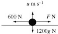
Let the speed of the car be  $u \text{ m s}^{-1}$  and the driving force of the engine have magnitude  $F \text{ N}$ .
