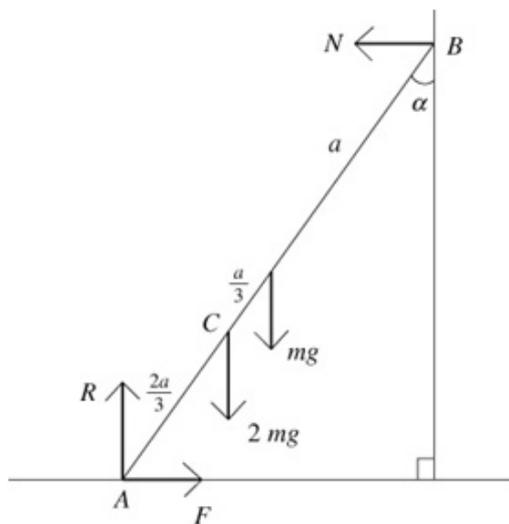
Let  $N$  be the force between the ladder and the wall at  $B$  – perpendicular to the wall since no friction here. Let  $R$  be the normal reaction at  $A$ , and  $F$  the friction at  $A$ .
