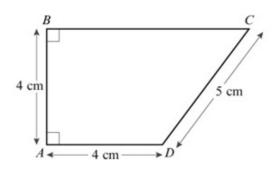
A thin uniform wire of total length 20 cm, is bent to form a frame. The frame is in the shape of a trapezium ABCD, where AB = AD = 4 cm, CD = 5 cm and AB is perpendicular to BC and AD, as shown in the figure.
