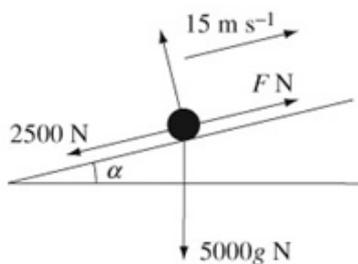
Let  $F\text{N}$  be the magnitude of the driving force produced by the engine.
