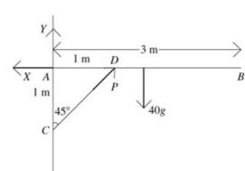
Let the horizontal and vertical components or the force at A be X and Y respectively. Let the thrust in the rod be P.
