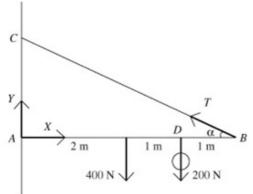
Let the tension in cable *BC* be *T*. The horizontal and vertical components of the tan  $\alpha = \frac{1}{2} \Rightarrow \sin \alpha = \frac{1}{\sqrt{5}}$  reaction at *A* are *X* and *Y* respectively.
