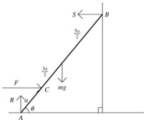
Let  $S$  be the force between the ladder and the wall at  $B$ .
