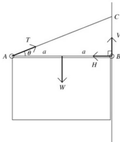
$T$  is the tension in the string,  $V$  and  $H$  are horizontal and vertical components of the force at  $B$ .
