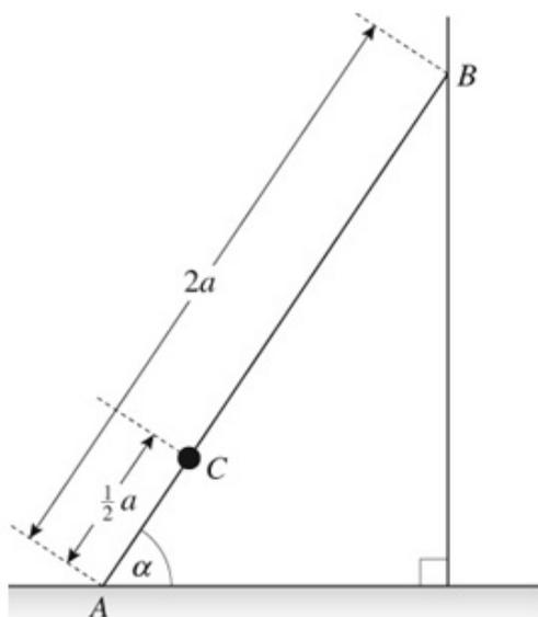
A uniform ladder  $AB$ , of mass  $m$  and length  $2a$ , has one end  $A$  on rough horizontal ground. The other end  $B$  rests against a smooth vertical wall. The ladder is in a vertical plane perpendicular to the wall. The ladder makes an angle  $\alpha$  with the horizontal, where  $\tan \alpha = \frac{4}{3}$ . A child of mass  $2m$  stands on the ladder at  $C$  where
