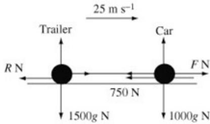
Let  $F$  N be the magnitude of the driving force produced by the engine of the car.
