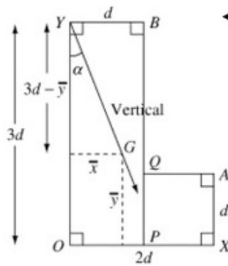
You divide the L-shaped lamina into parts, each with a known centre of mass. This can be done in different ways. Here the lamina has been divided up into a rectangle  $OYBP$  of dimensions  $3d \times d$  and a square  $AXQP$  of side  $d$ .
