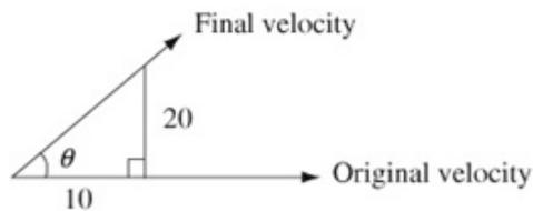
$$\begin{aligned} \tan \theta &= \frac{20}{10} \\ \theta &= 63.4^\circ \end{aligned}$$
