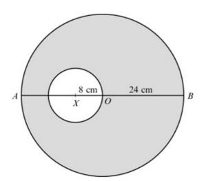
The figure shows a template T made by removing a circular disc, of centre X and radius 8 cm, from a uniform circular lamina, of centre O and radius 24 cm. The point X lies on the diameter AOB of the lamina and AX = 16 cm. The centre of mass of T lies at the point G.
