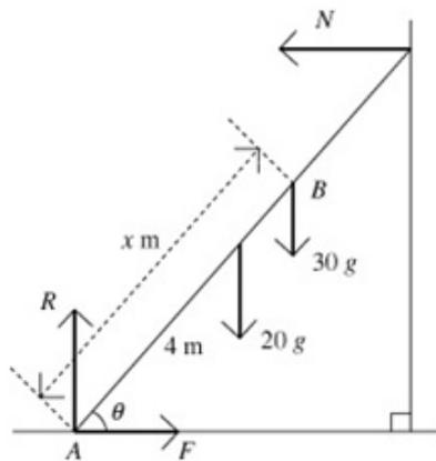
Suppose that the boy reaches the point  $B$ , distance  $x$  from  $A$ , the end of the ladder in contact with the ground.
