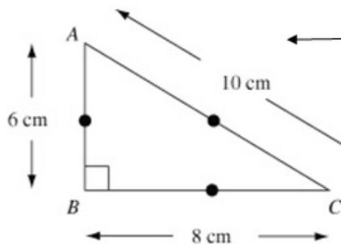
When there is no diagram, it is a good idea to sketch one. You are expected to recognise that a triangle with sides in the ratio of 3 : 4 : 5 has a right angle.
