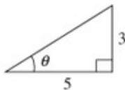
$$\begin{aligned} \tan \theta &= \frac{3}{5} \\ \theta &= 31^\circ \text{ (nearest degree)} \end{aligned}$$
