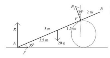
N is the normal reaction at P, R is the normal reaction at A and F is the friction at A.
