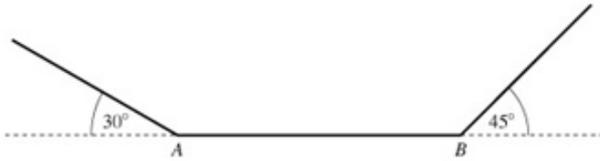
A non-uniform rod  $AB$  of mass  $5\text{ kg}$  and length  $4\text{ m}$ , with a particle of mass  $2\text{ kg}$  attached at  $B$ , rests horizontally in equilibrium supported by two strings attached at the ends of the rod.
