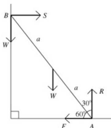
Adding the load at the top of the ladder and using the limiting equilibrium:
