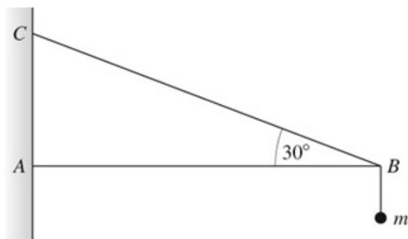
A uniform rod  $AB$  has mass  $2m$  and length  $a$ . The end  $A$  is smoothly hinged at a fixed point. A particle of mass  $m$  is suspended from the rod at the end  $B$ . The loaded rod is held in equilibrium in a horizontal position by a light string, one end of which is attached to the rod at  $B$ , the other end being fixed to a point  $C$  vertically above  $A$ , as shown in the diagram. The string makes an angle of  $30^\circ$  with the horizontal.
