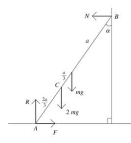
Let N be the force between the ladder and the wall at B- perpendicular to the wall since no friction here. Let R be the normal reaction at A, and F the friction at A.
