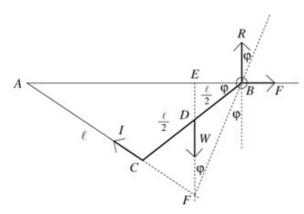
The diagram of forces has four forces acting, the weight, W, the tension, T, in the cord, the normal reaction, R, and the friction, F, at the ring end. Combining R and F to give a single contact force at the ring reduces the problem to one of an object in equilibrium with three forces acting. These must be concurrent.
