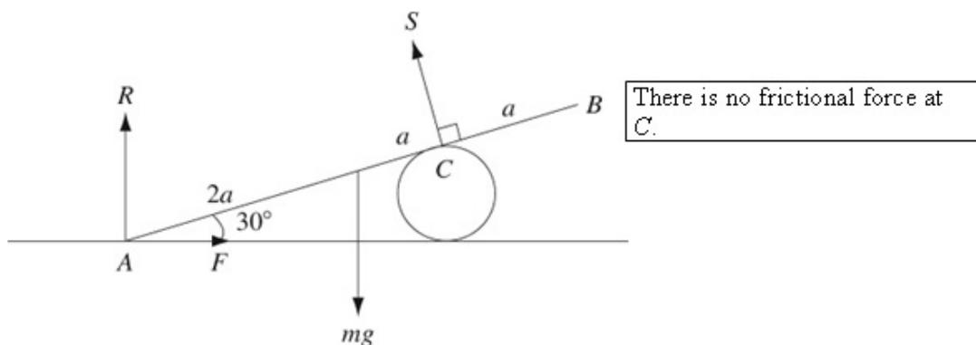
**a**  $M(A) \quad S \times 3a = mg \times 2a \cos 30^\circ$
