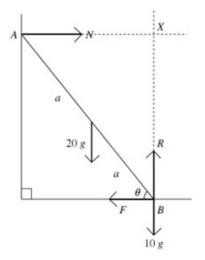
Let the ladder have length 2a, and be inclined at  $\theta$  to the horizontal.
