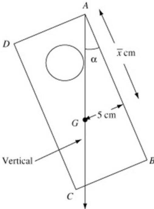
When the plate is suspended freely from  $A$ , its centre of mass  $G$  is vertically below the point of suspension  $A$ . The distance of  $G$  from  $AD$  was found in **a** and the distance of  $G$  from  $AB$  is 5 cm by symmetry. You calculate  $\alpha$  using trigonometry.
