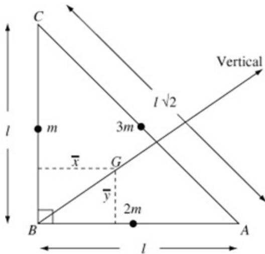
As  $l^2 + l^2 = (l\sqrt{2})^2$ , the angle at  $B$  is a right angle.
