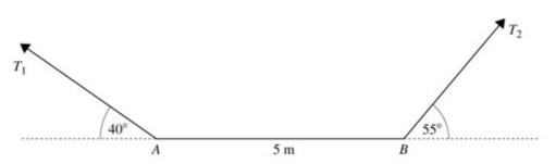
A uniform rod AB of mass 3 kg and length 2 m rests horizontally in equilibrium supported by two strings attached at the ends of the rod. The strings make angles of 40° and  $\theta$  with the horizontal, as shown in the diagram. Find the magnitudes of the tensions in the strings and the value of  $\theta$ .
