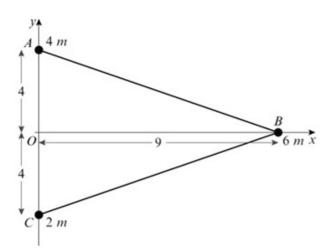
The figure shows a triangular lamina ABC. The coordinates of A, B and C are (0, 4), (9, 0) and (0, -4) respectively. Particles of mass 4m, 6m and 2m are attached at A, B and C respectively.
