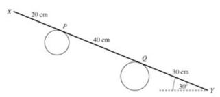
A uniform rod XY has weight 20 N and length 90 cm. The rod rests on two parallel pegs, with X above Y, in a vertical plane which is perpendicular to the axes of the pegs, as shown in the diagram. The rod makes an angle of 30° to the horizontal and touches the two pegs at P and Q, where XP = 20 cm and XQ = 60 cm.
