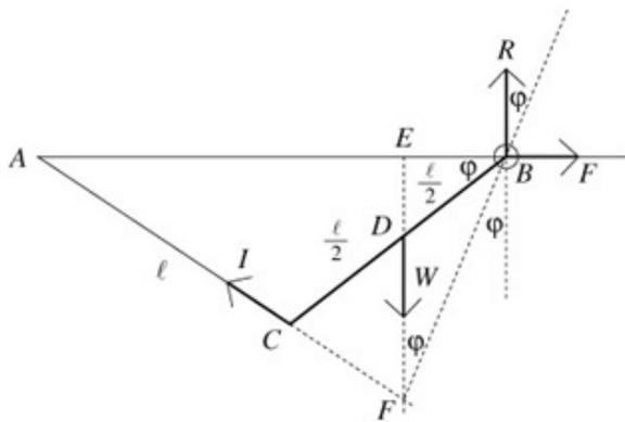
The diagram of forces has four forces acting, the weight,  $W$ , the tension,  $T$ , in the cord, the normal reaction,  $R$ , and the friction,  $F$ , at the ring end. Combining  $R$  and  $F$  to give a single contact force at the ring reduces the problem to one of an object in equilibrium with three forces acting. These must be concurrent.
