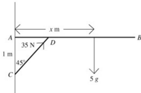
Suppose that the centre of mass is  $x\text{ m}$  from  $A$ . We are not told anything about any force(s) acting at  $A$ , but as they have zero moment about  $A$  this will not matter.
