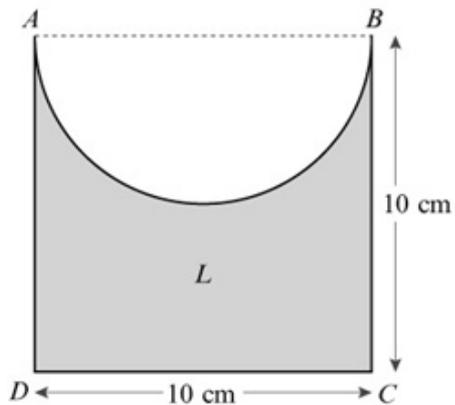
A uniform lamina  $L$  is formed by taking a uniform square sheet of material  $ABCD$  of side 10 cm and removing a semicircle with diameter  $AB$  from the square, as shown in the figure.
