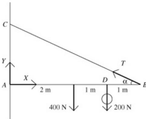
Let the tension in cable  $BC$  be  $T$ . The horizontal and vertical components of the  $\tan \alpha = \frac{1}{2} \Rightarrow \sin \alpha = \frac{1}{\sqrt{5}}$  reaction at  $A$  are  $X$  and  $Y$  respectively.
