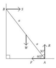
Let A and B be the ends of the ladder. S is the normal reaction at B, R the normal reaction at A and F the friction at B. The length of the ladder is 2a. **a**
