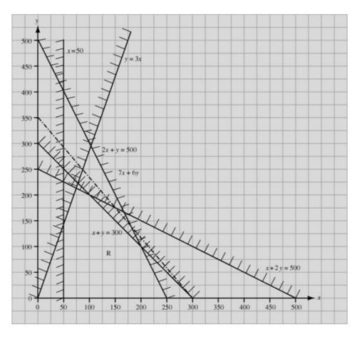
Objective line passes through (0, 350) and (300, 0). Maximum point is (200, 100). P = 2000.
