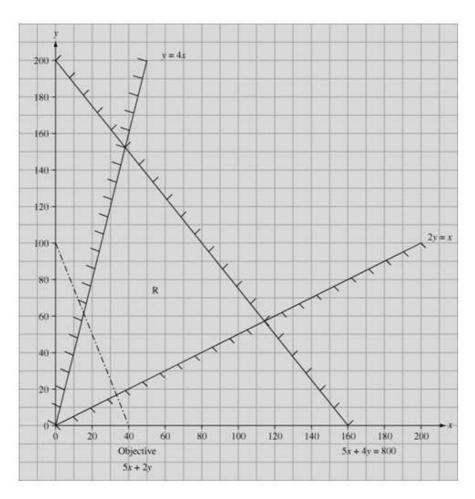
Solving 2y = x and 5x + 4y = 800 simultaneously gives  $\left(114\frac{2}{7}, 57\frac{1}{7}\right)$  Test integer values nearby.
